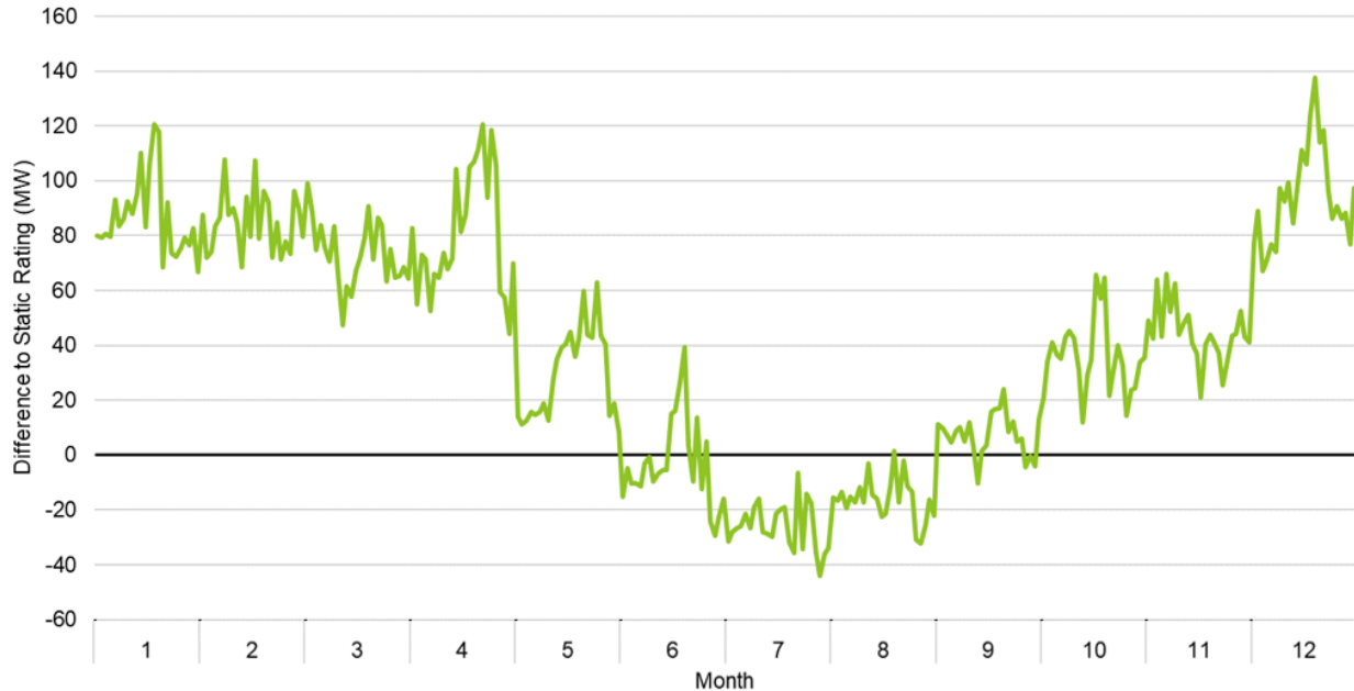
Figure 19. Change to dynamic line rating relative to static line rating for Canandaigua to Avoca 230-kV line.
